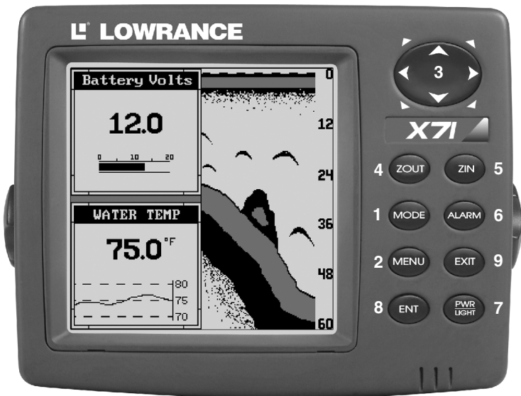
Lowrance X71 Sonar, front view, showing screen and keyboard.
